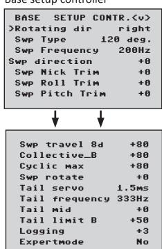
When a value is activated in the basic setting control, the gyro control and partly the control are deactivated! Therefore, settings must not be carried out in the air, but must be carried out on the ground without speed!
