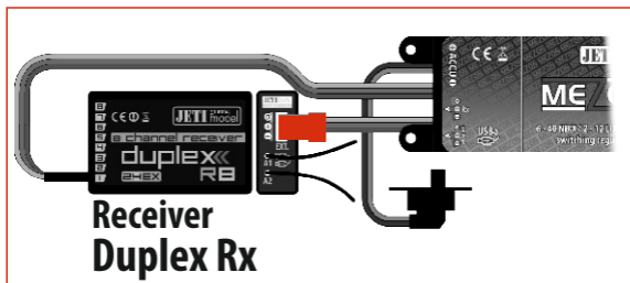
Fig. 5: Connection for the MEZON telemetry.
